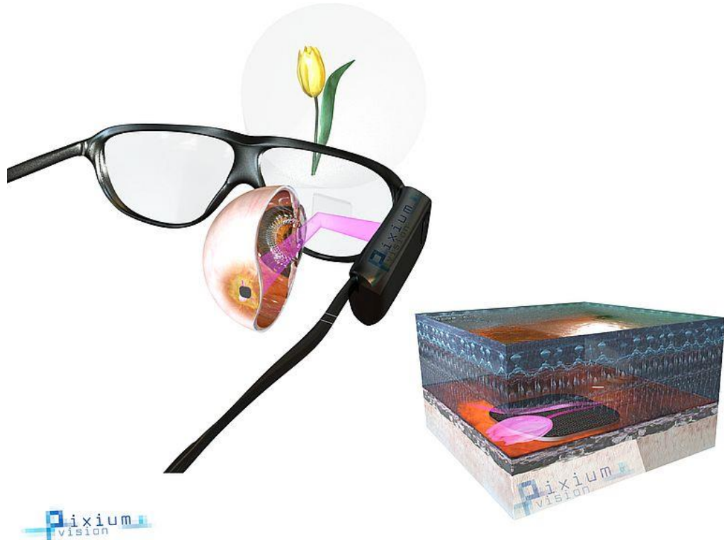
Exhibit 1: Diagram of Prima including camera integrated into specialised glasses
