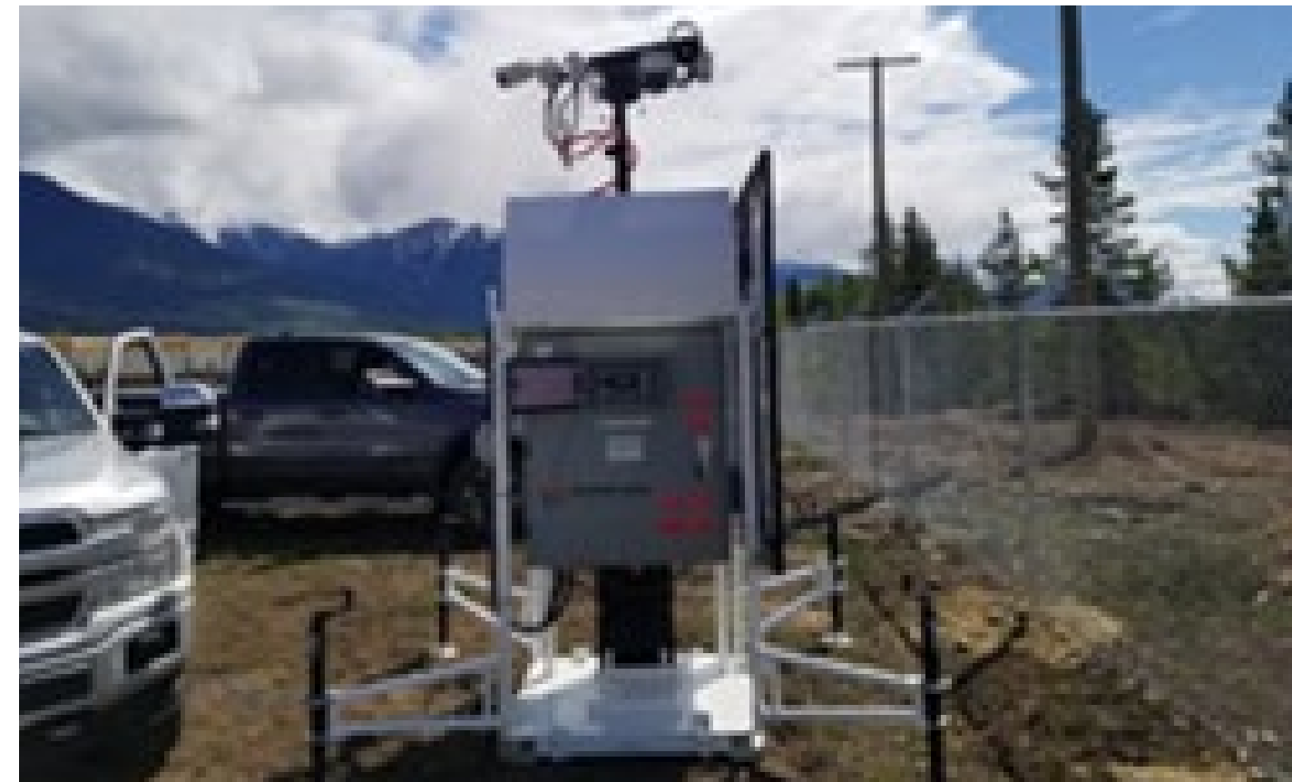
Exhibit 24: Autonomous off-grid hybrid power for remote video surveillance equipment (direct methanol fuel cell)
